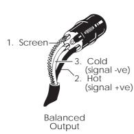
The left and right main outputs are on 3-pole male XLR connectors, wired as shown on the left. They are balanced outputs, allowing long cable runs to balanced amplifiers or other equipment. If the amplifier (or other equipment) which you are using has an unbalanced input, you should wire the output from the D-MIX500 as shown in the 'Balanced To Unbalanced' diagram below.
